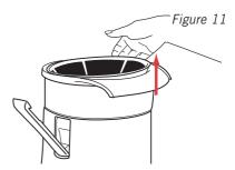
6. Lift the juice collector/bowl from the motor base – figure 12.
